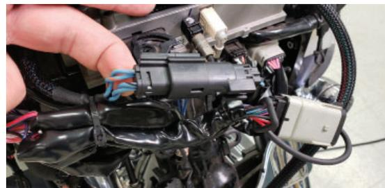
3. Route the harness along the clutch side to the rear pods; notice the tags for the clutch side and the throttle side.
