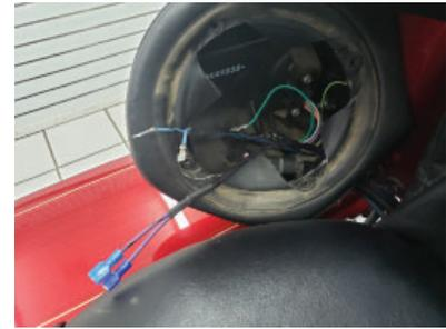
8. Connect the speaker wires to the factory or replacement speaker and connect the input wires to the factory speaker wires. Use shrink wrap over the connections to factory speaker wires to avoid shorts.
